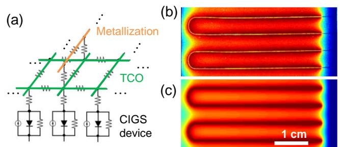
Fig. 1. (a) schematic of the distributed-element circuit analysis approach for optimizing metallization and TCO design. (b) Measured and (c) simulated electro-luminescence images from a solar cell of interest.
