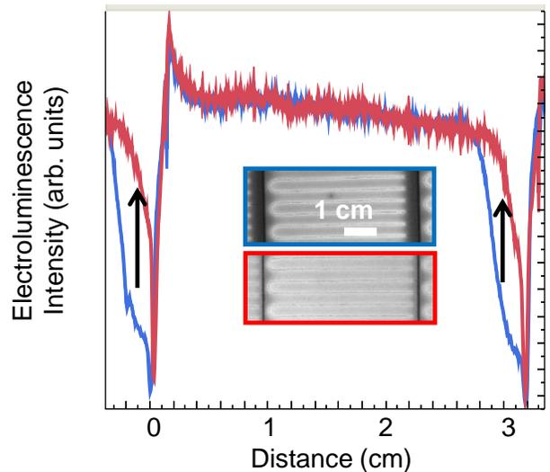
Fig. 4. Measured electroluminescence (EL) line scans and images from baseline (blue) and experimental (red) cell integration designs, where the experimental cell interconnect shows increased EL intensity at the cell edge.
