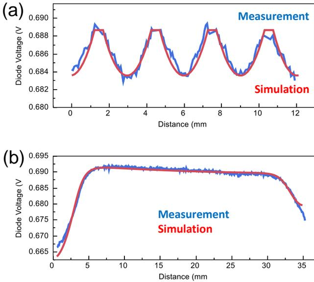
Fig. 2. Electroluminescence (EL) line scan overlays based on the images from Fig. 1b and 1c. Both (a) vertical and (b) horizontal EL line scans show the close correspondence between measurement and simulations.
