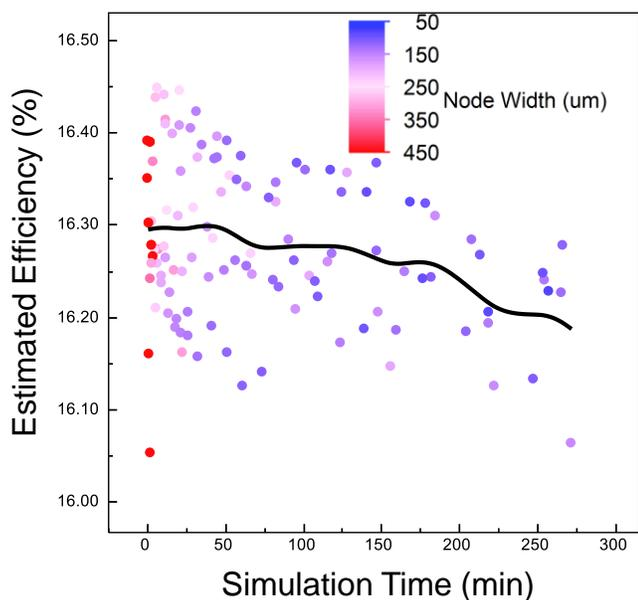
Fig. 6. Scatter plot showing estimated device efficiency results for a range of simulation node width values. The standard deviation in estimated device efficiency is found to decrease with smaller node size. Simulations with node width values <200 μm were found to provide efficiency estimates with a standard deviation value <0.05% abs.
