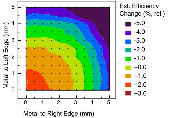
Fig. 3. Contour map showing simulation results for a range of cell integration geometries. The highest performance is expected for smaller “Metal to Edge” distances. “Left” and “Right” are based on the orientation of the solar cells shown in Fig. 1b,c.
