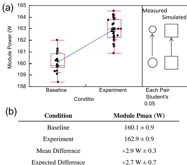
Fig. 5. Module power results from the comparison of baseline and experimental cell interconnect designs. Experimental cell interconnect design shows +2.9 W (+1.8% relative) mean module power improvement.
