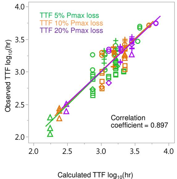
Figure 1: Observed and calculated time-to-failure (TTF) data under damp heat conditions for c-Si solar cells in a glass-polymer package with EVA encapsulant. The marker shape represents the data source as follows:  $\diamond$  [7],  $+$  [8],  $\Delta$  [9],  $\circ$  [10],  $\square$  this paper. The time to failure data is fit to the power law relation,  $t_{TTF} = A * e^{(E_a/kT)} * RH^n$ , where  $E_a = 0.89$  eV, and  $n = -2.2$ .
