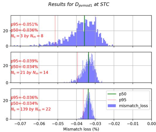
Fig. 4. Distribution of STC mismatch losses at various system scales for  $D_{pvmod1}$
