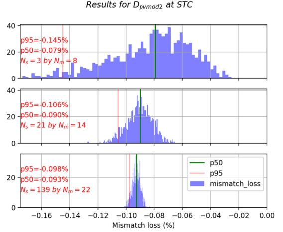
Fig. 5. Distribution of STC mismatch losses at various system scales for  $D_{pvmod2}$
