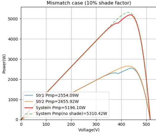
Fig. 1. Power-Voltage curve of a 2x10 PV system – 1st module in String 1 shaded 10%, shading mismatch loss = -0.4%
