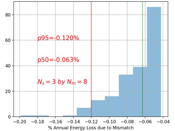
Fig. 6. Example of distribution of Annual Energy Loss due to Mismatch for a typical  $N_s=3$  by  $N_m=8$  using dataset  $D_{pvmod1}$
